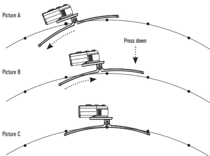
**Do not bend bracket, as it could cause bracket to deform or break!**
